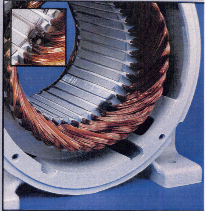
6 Winding Grounded at Edge of Slot
